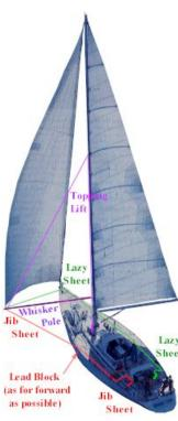
Whisker poles are designed to operate under higher compressive forces than spinnaker poles. Since tube diameter and wall thickness are a major function of strength, whisker poles must be sized accordingly. The size requirement of the whisker pole depends on boat length, type of sail used and general wind conditions. Additional variables include displacement and bow sprits that extend the basic fore-triangle.
