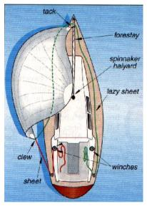
The cruising spinnaker does not require a spinnaker pole
