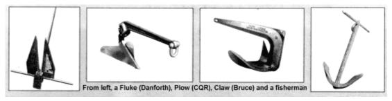
**Danforth anchors:** The lightweight anchor, such as the Danforth or Fortress, is a burying anchor with wide sharp flukes and a stock. It holds very well under high loads in mud and sand but may be difficult to set in clay, grass, weeds, rock or shell bottoms. You may want to consider a lightweight as a secondary working anchor or a lunch hook. It requires more scope than other anchors and can be stored flat on deck, or from a rail.
