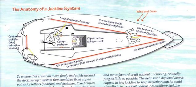
points should be installed near the helm, winches, companionway, and foredeck. Jacklines should be taut and allow the crew to clip in from the safety of the cockpit
