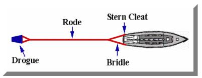
attached to a rode. The rode is then attached to a bridle (a line running from one port winch or cleat, into the water behind the stern and attached to the starboard winch or cleat.) A bridle will reduce the load on a cleat or winch by distributing the force between both the port and starboard sides of the boat.
